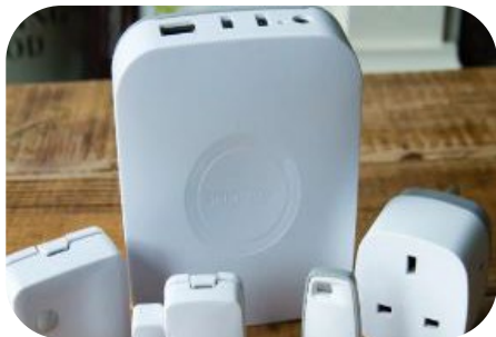
Hub and sensors (Water, Fire, Temp, Motion)
