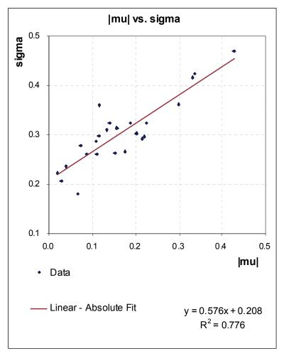
The  $\sigma$  parameter can be approximated as a function of the  $\mu$  parameter
